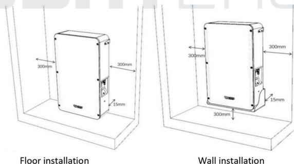
If the battery is installed indoors, please leave a certain gap during installation according to the picture above, ventilation is required, combustible materials should not be placed around the battery.
