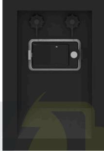
2. Press the battery power button, the power button LED light is on, and 2 LED indicator lights will be on and show the green color after self-check.
