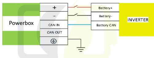
Overcurrent and disconnection protection device must be installed between the battery and the inverter that isolates both positive and negative conductors.
